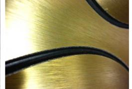
For accurate and precise manual folding of the Alupanel composite panels, resulting in a good finish, we recommend to route the rear of the panels to 2.5 mm thick, going through the exterior Aluminium layer, and some of the Polyethylene core. Normally the panel is grooved and folded 25-70 mm from the edge.
